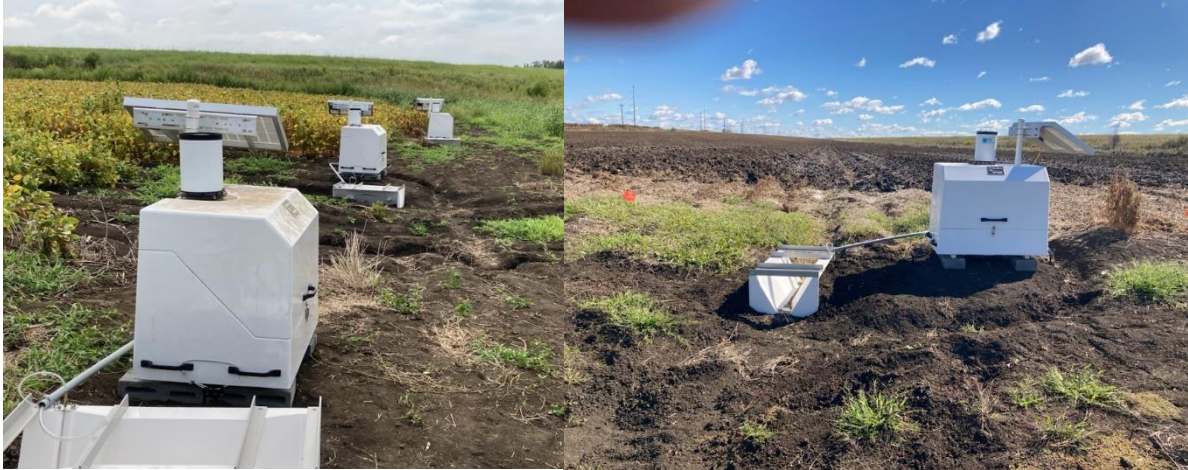
Fig. 4. Five automatic runoff collectors (ISCO Inc., Lincoln, NE) as shown below were installed at the edge of a soybean field at Good Farm, Noxubee County, MS.
