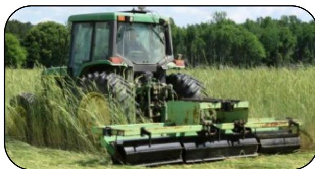
Straight crimping bar roller/crimper
