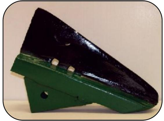
**Splitter points** help prevent soil blow-out, especially in dry soils. Newer shanks may incorporate this design, or a piece of metal can be welded perpendicular to the center of a subsoiler shank tip.
