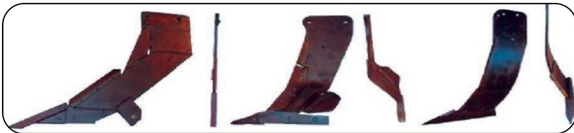
Side and front view of an in-row subsoiler (left) and two bent-leg subsoilers.
