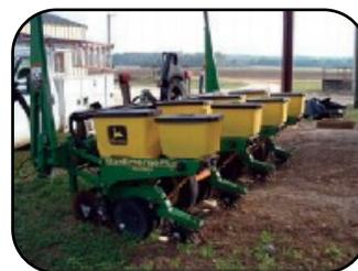
Most planters and drills used in conservation systems have coulters in front of the seed openers to help cut through heavy residue. There are several different coulters available.
