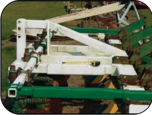
**Toolbar extensions** on older subsoilers can help ensure that the coulter is running on firm ground ahead of the shank to help cut residue.
