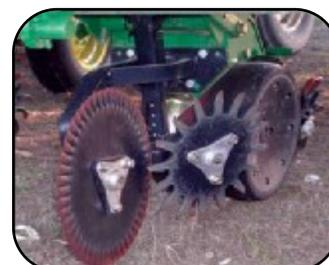
**Double disk openers** create a slot for seed placement. Notched openers can help move residue away from the seedbed to prevent hairpinning.
