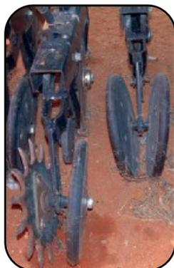
**Down-pressure springs** maintain the desired seeding depth in high residue or on uneven and/or firm ground.
