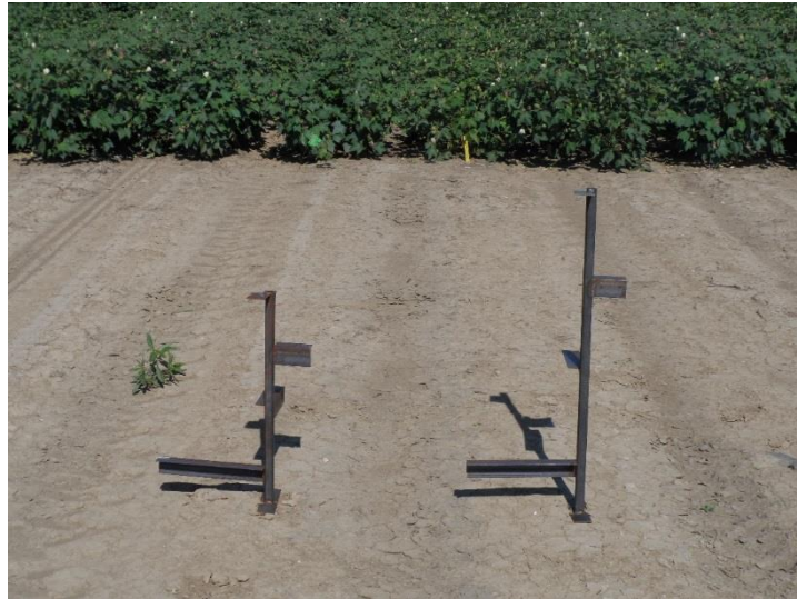
Figure 4. Metal stands used to determine impact of deposition aids on pesticide deposition into the soybean canopy.
