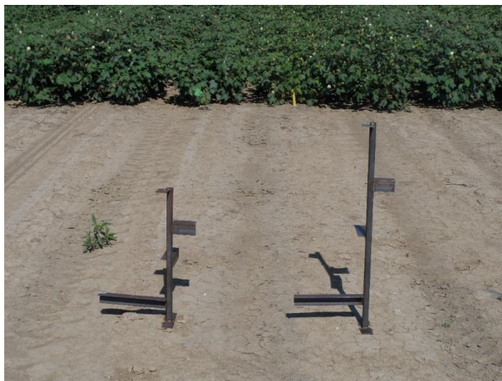
Figure 1. Metal stands used to determine impact of deposition aids on pesticide deposition into the soybean canopy.
