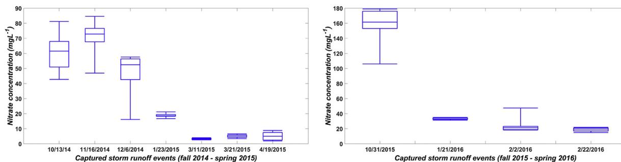
Fig. 2. Nitrate concentration in individual storm runoff events captured from fall 2014–spring 2015 (left) and fall 2015–spring 2016 (right).
