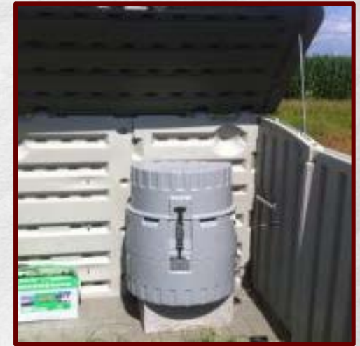
ISCO 6712 portable sampler for collecting runoff samples.
