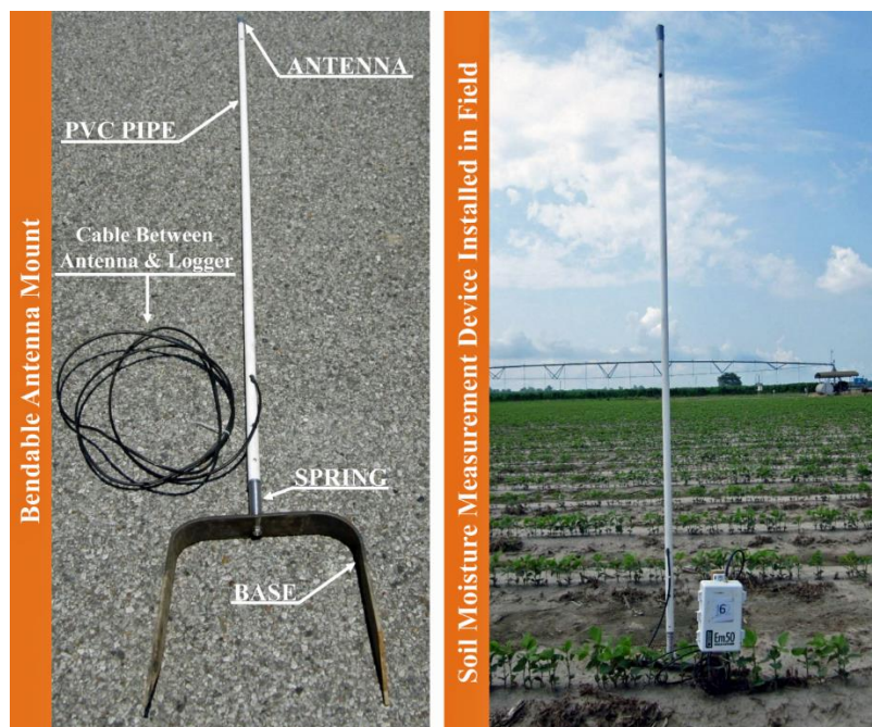
Fig. 1. Bendable antenna mount (left) and soil moisture sensing device with a bendable antenna mount installed in a soybean field for irrigation scheduling (right).
