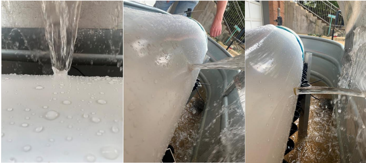
Figure 1. Turbulent water flow from Poly Piranha II (left, center) vs. mechanically inserted hole (right).
