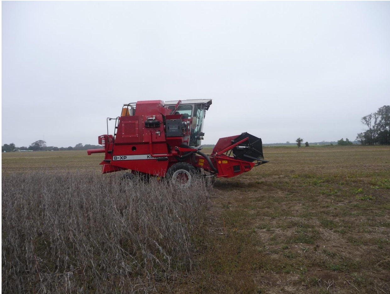
Figure 9. A two-row harvester equipped with a load cell, allowing collection of yield data per each treatment. The picture was taken on October 27, 2020. Cultivar was P46A57BX.
