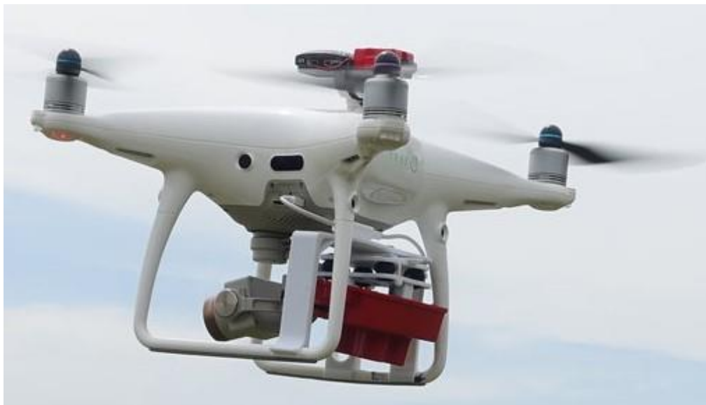
Fig. 2. MicaSense RedEdge-M camera and companion DLS and GPS units (b) Parrot sequoia camera and companion sunshine sensor with GPS.
