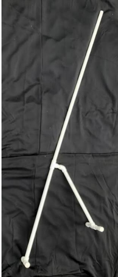
Figure 1.2 PVC structure which held camera at consistent position and height above crop canopy.
