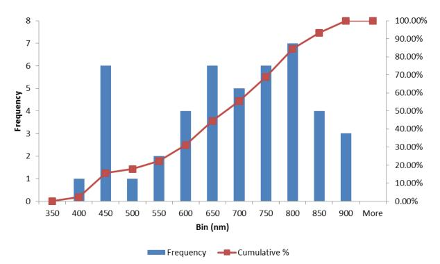
The graphs show the wavelength distribution for detection of GR and GS Italian ryegrass and the principal bands are around 450 nm, 650 nm and 800 nm. This formation is important for us to simplify the sensor system to develop a portable device for farmers to use in the field, with further validation through meta-analysis of more band selection data.
