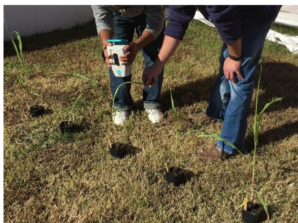
Figure 2. ASD hyperspectral measurement of greenhouse-grown Johnsongrass under the sun light.
