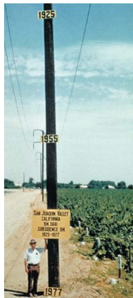
Figure 9. Land subsidence in San Joaquin Valley, California (Galloway, Jones, and Ingebritsen 1999). The person standing by the post in the photo is Dr. J. F. Poland.
