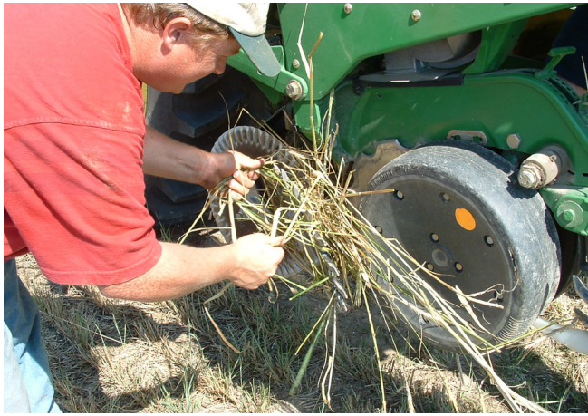
Figure 6. Removing residue that becomes entangled in equipment can waste considerable time, leading to grower frustration with cover crops. Photo courtesy of Ted Kornecki, USDA-ARS.
