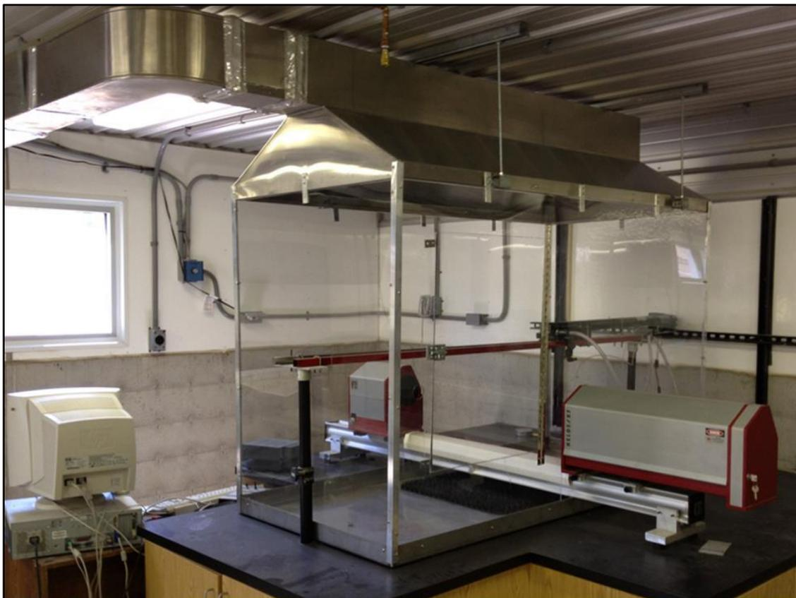
Figure 2.1. Static chamber and Sympatec laser diffraction system used to characterize sprays of 720 treatment combinations.
