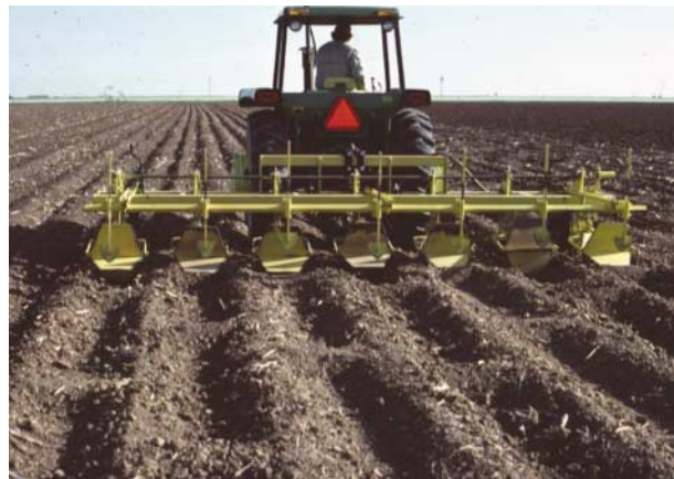
Fig. 2 The most common type of furrow diker is the tripping paddle type, which is often used concurrently with cultivation of ridge till fields after planting.
