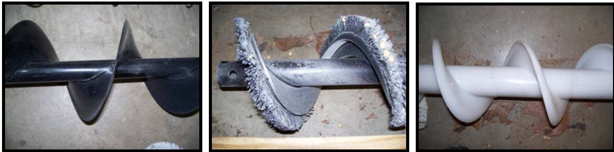
Figure 1: Section pictures of steel, brush, and plastic cupped auger designs.
