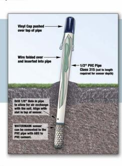
Automatic Data Collection systems provide a graphical record of soil moisture trends to assist the grower in making critical irrigation scheduling decisions. The equipment is simple to install and use. Designed for harsh outdoor installations, all our enclosures are weather tight. WaterGraph software is included and takes only a few minutes to set
