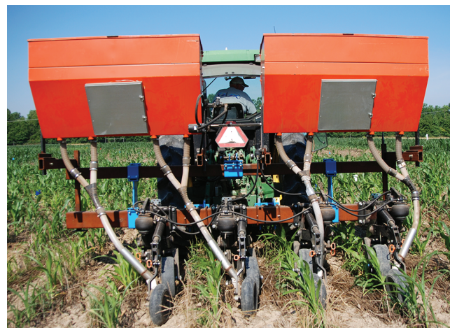
Fig. 1. Prototype subsurface banding applicator used to sidedress pelletized poultry litter.
