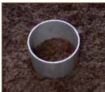
Figure 7. Ring driven to 3-inch depth.
