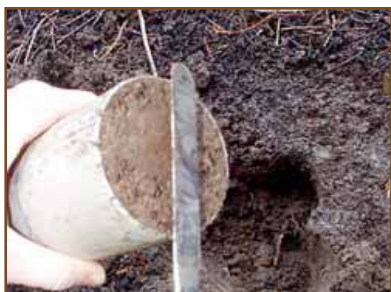
Figure 8. Remove excess soil from bottom of ring.
