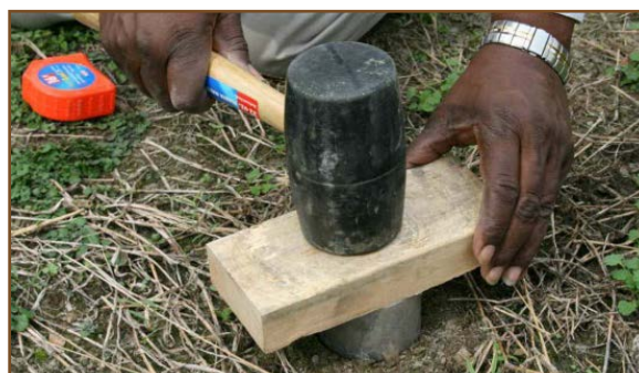
Figure 6. Drive ring to 3-inch depth.
