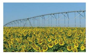
[LESA] and low energy precision application [LEPA] have been added to center pivot machines to apply water very close to or on the soil surface of the field to improve application efficiency.
