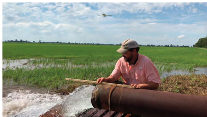
Photo 10-1. Manual measurement of pump flow using a yardstick and plumb bob.
