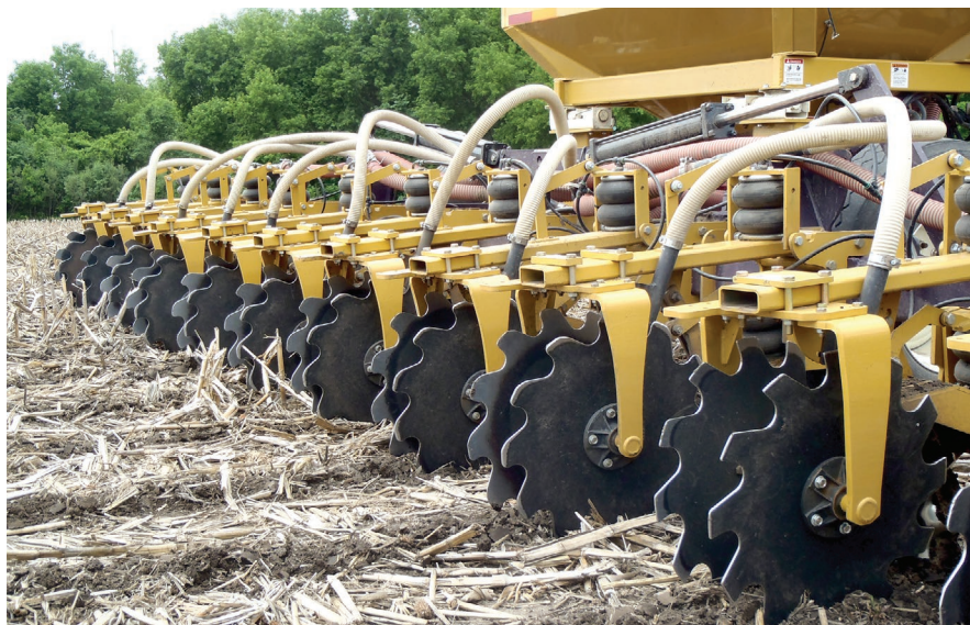
With reduced-tillage practices, such as strip tillage shown here, soil structure improves, allowing greater plant-available water storage, improved root exploration, improved cycling of organic matter, and improved timing/efficiency of plant-available nutrients. Photo courtesy of Flickr/MPCA Photos.
