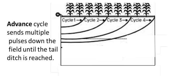
Surge Valves are being investigated by the MSU Irrigation Team to increase irrigation application efficiency. When using a surge valve, water is applied in a series of on-off cycles alternating between two irrigation sets. By utilizing surge valves Producers can expect reduced surface runoff, reduced deep percolation loss, and application inefficiencies 25% great than conventional irrigation techniques. In sealing silt loam soils improved infiltration rates have been documented.
