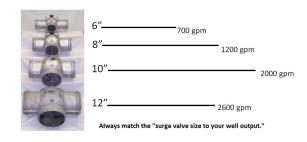
Based on the chart to the right, a 6" surge valve has a capacity from 0 to approximately 700 GPM while the much larger 12" will handle well capacities up to 2600 GPM.
